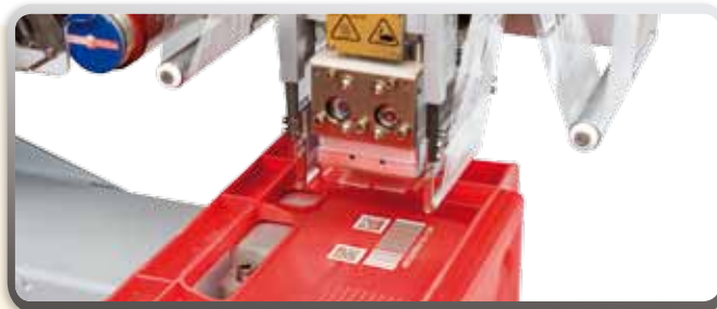
Printing on containers and boxes in recesses up to 20 mm deep.
