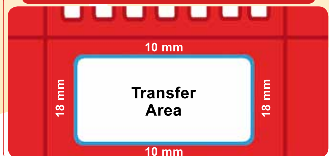
Definition of the minimum side margins between the writing and the walls of the recess.
